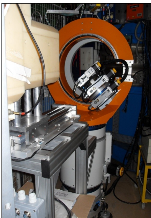
Figure 2: Sample-detector support with a new Euler Cradle including x,y,z translations.
